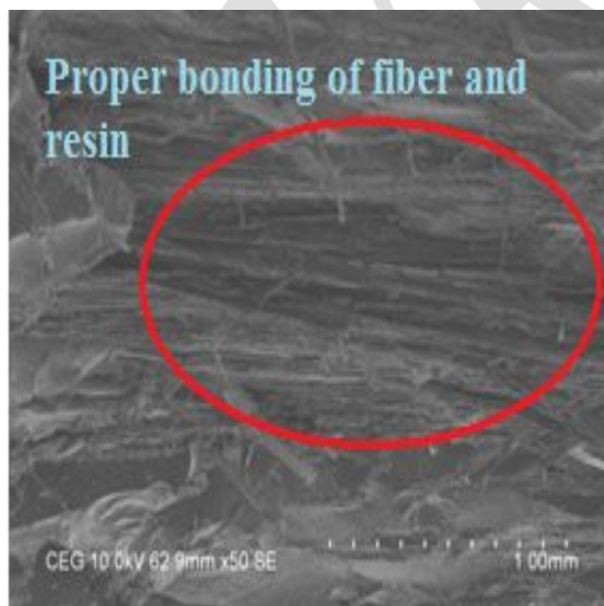
Figure 7 SEM image 100% jute fiber reinforced composite after tensile test
